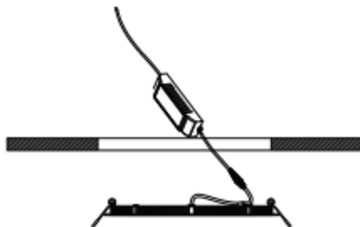
2a Connect PSU Mains AC Cable 2b PSU /Downlighters DC cables
